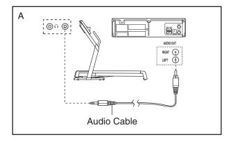
B. Plug one end of a long 1/8" to RCA stereo audio cable (available at electronics stores) into the input jack on the console. Plug the other end of the cable into an RCA Y-adapter (available at electronics stores). Next, remove the wire that is currently plugged into the AUDIO OUT jack on your VCR and plug the wire into the unused side of the Y-adapter. Plug the Y-adapter into the AUDIO OUT jack on your VCR.
